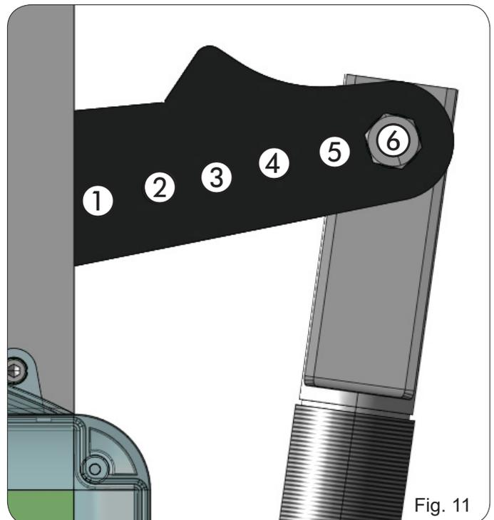
The following two tables indicate the fixing position of the pistons on the rocker arm in relation to the length of the beam and the presence of accessories secured to it, if any.
